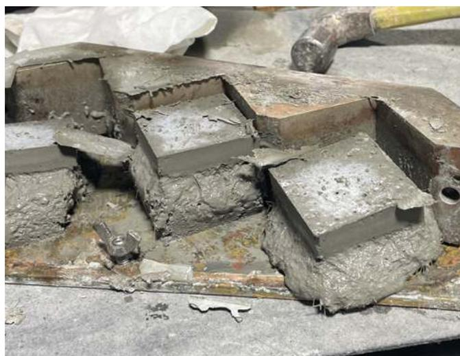
Fig. 7: UHPC cured slowly in a cold temperature environment (picture taken 24 hours after placement). Ambient curing temperature was estimated to be 55°F (13°C)
