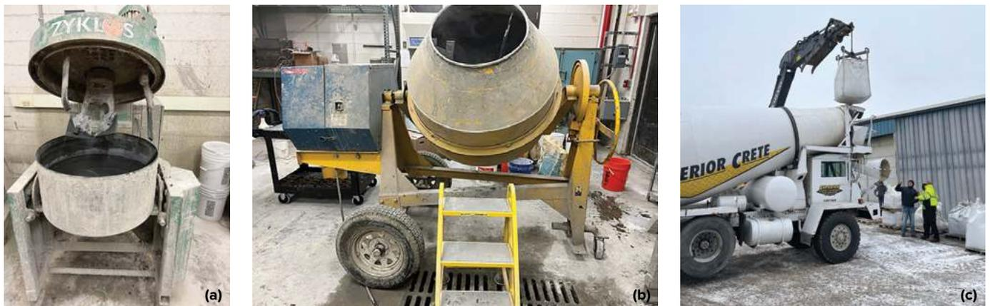
**Fig. 5:** Types of mixing equipment used in this study: (a) rotating pan mixer (F1); (b) rotating drum mixer (F2); and (c) concrete truck (T)
