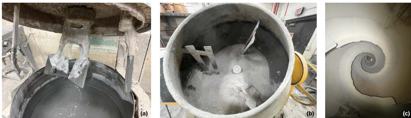
Fig. 6: Details of mixing equipment: (a) F1 mixer with side scrapers and high-shear “whirler” blades; (b) F2 mixer with fixed blades; and (c) T mixer with the spiral blade
