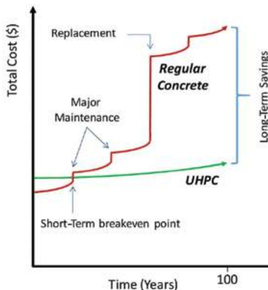
Fig. 5: Schematic diagram of life-cycle cost of UHPC and regular concrete
