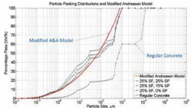
Fig. 2: Achieving high packing density in UHPC
